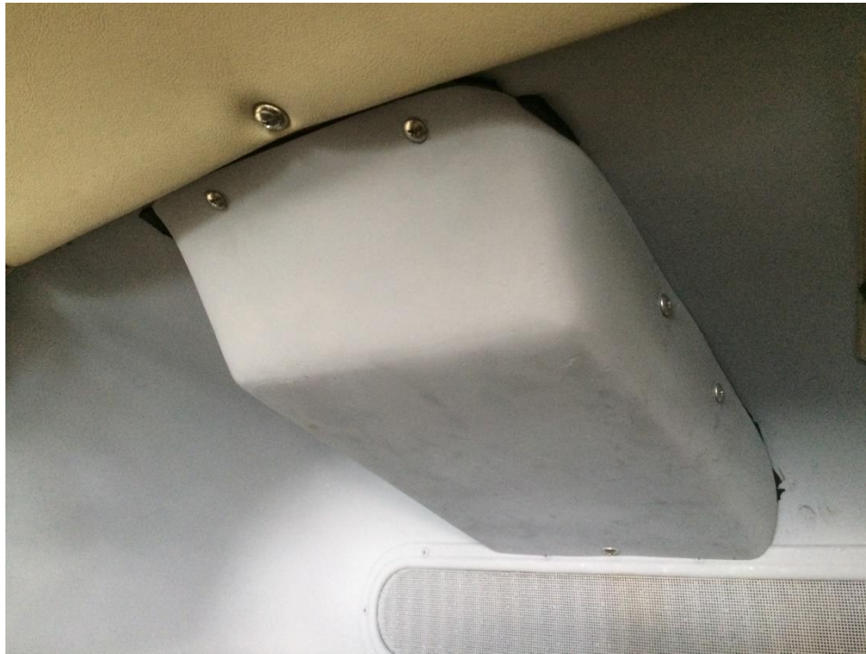
Figure 14 - Installed Duct Cover in Hat Shelf
