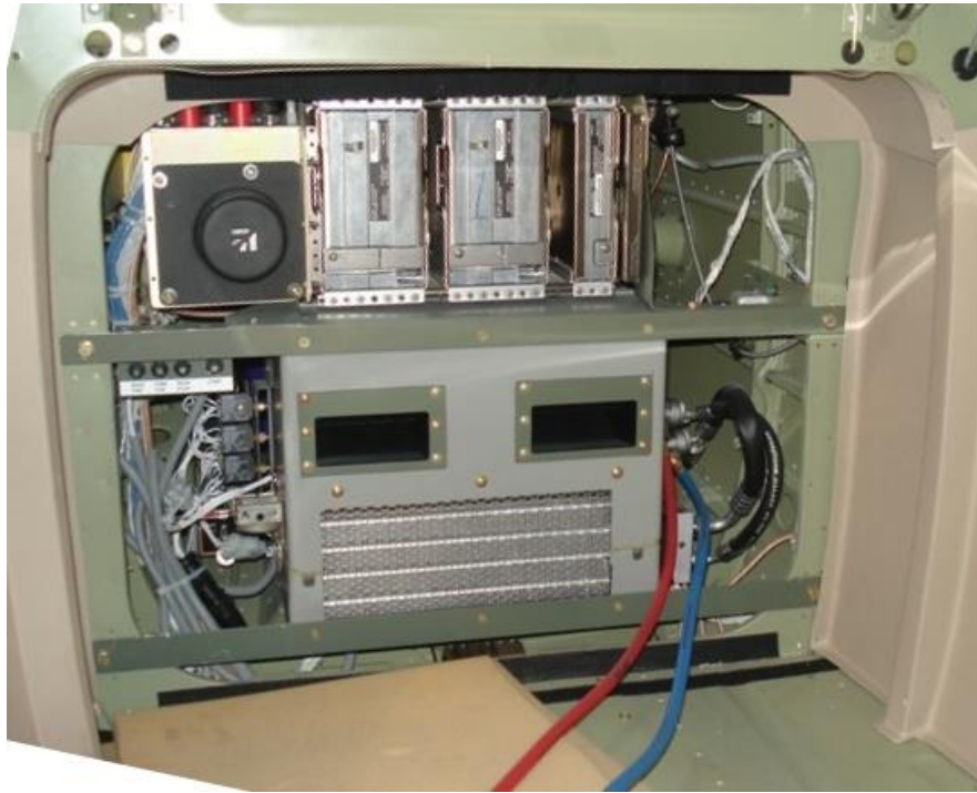
Figure 17 – Rear Evaporator Installation
