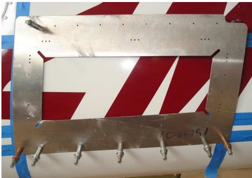
Figure 2 – 206 Port Reinforcement Template
