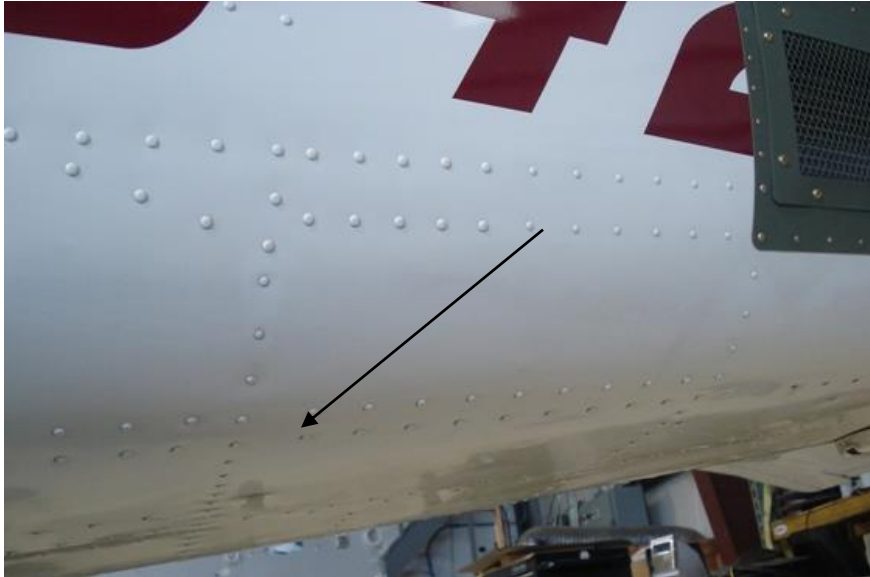
Figure 11 – Aft Evaporator Drain Location
