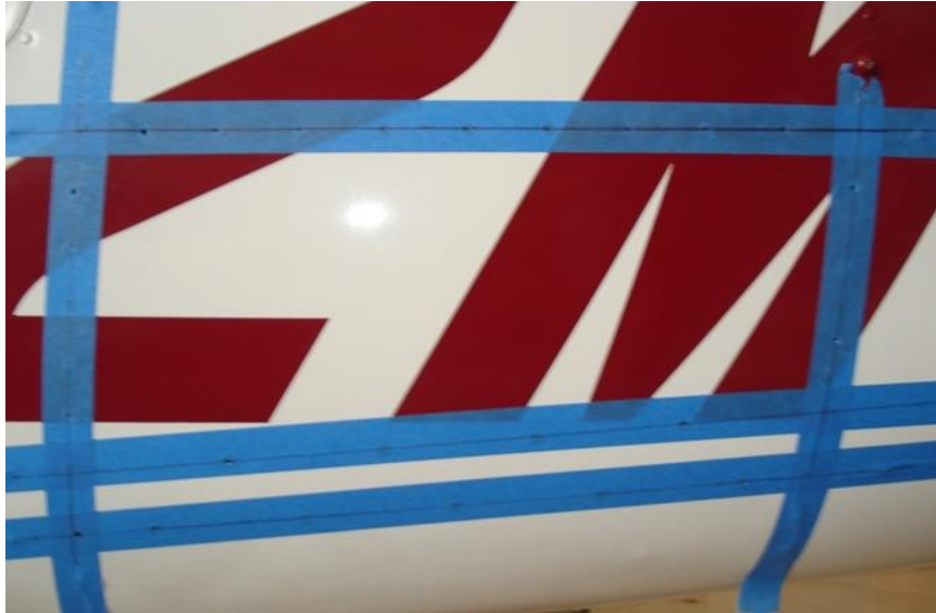
Figure 1 – Port Side Cutout Location
