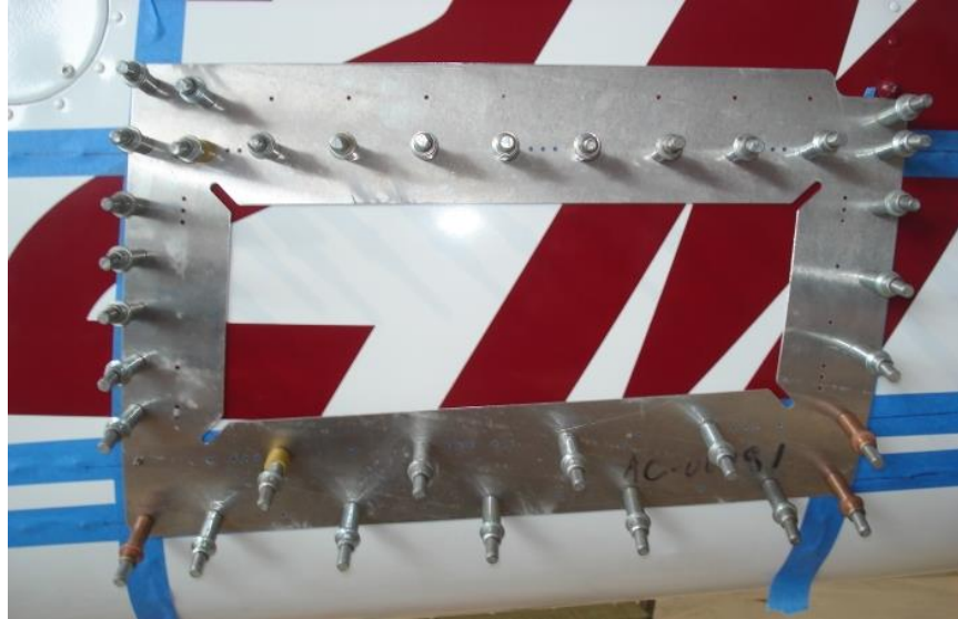
Figure 3 – 206 Port Reinforcement Template
