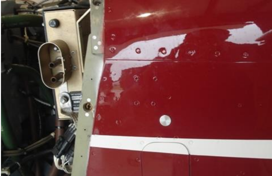
Figure 13 – Typical Piezo Electric Switch Installation
