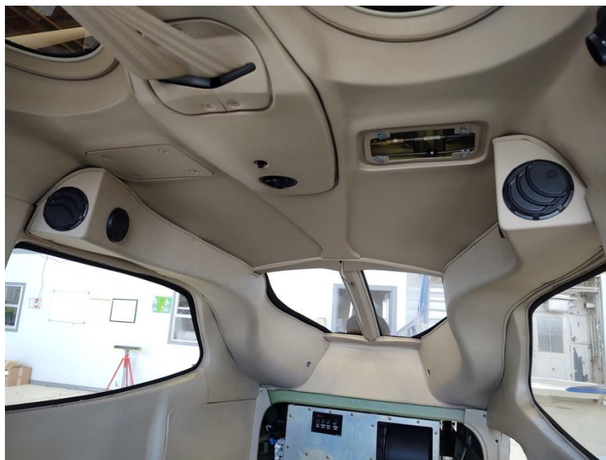
Figure 18 - Side Ducts Installed
